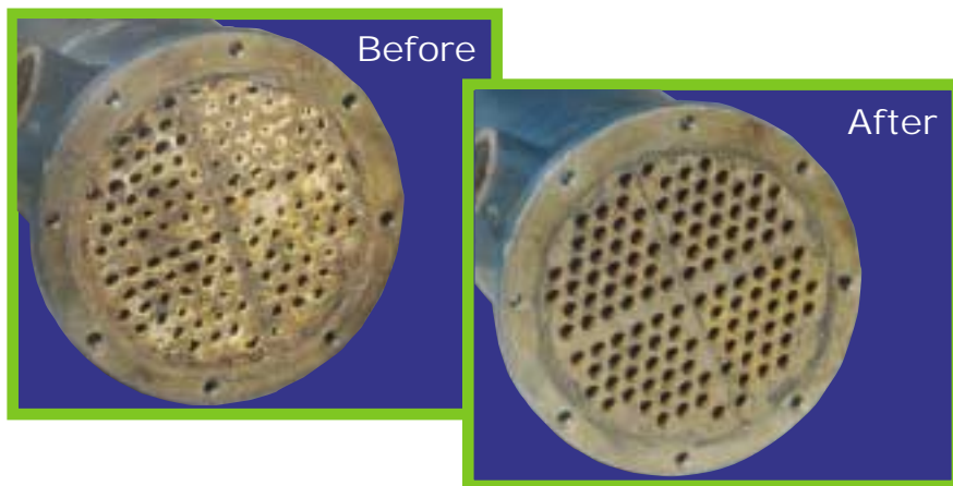
RYDLYME Marine restores efficiency on lube oil cooler.
