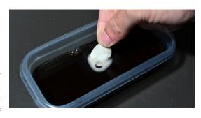
there is little or no reaction, the solution is expended. This test should be performed near the end of the recommended circulating time. If near the end of the recommended cleaning time the solution has been expended, more **RYDLYME Marine** will be required to complete the job. However, if the solution is still active at the end of the recommended time, all the scale has been dissolved within the
